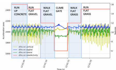
Figure 2. Time series example of the one-off activity “climb gate” versus repetitive data “run” and “walk”.
